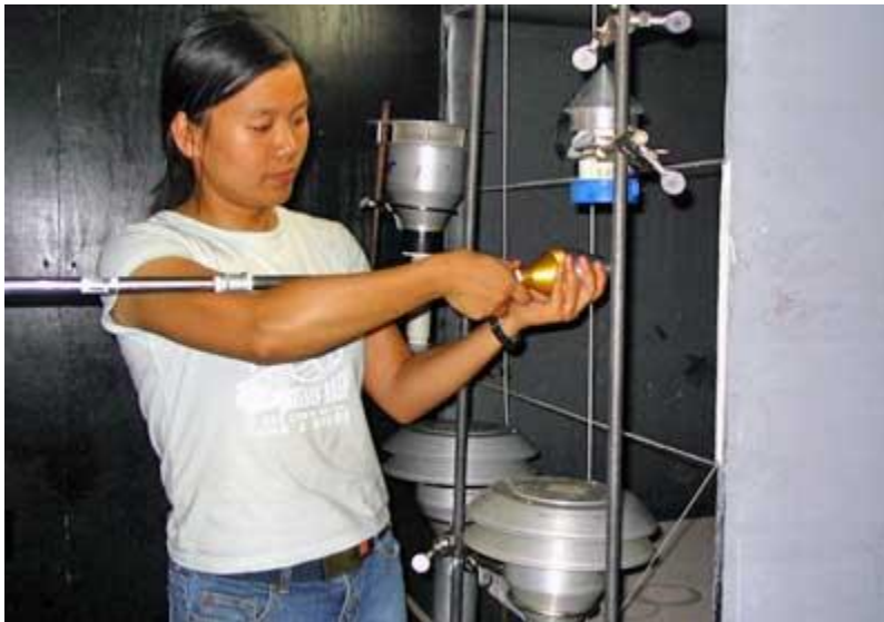
Jing Chen, graduate student, prepares FRM PM10 (particulate matter less than 10 micrometers) and TSP (total suspended particulate matter = 100 micrometers or less) sampler inlets for testing in a wind tunnel that allows for controlled PM concentration testing.
