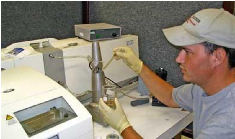
Kyle Kieschnick, student technician, performs a particle size distribution (PSD) using a Malvern Instruments Mastersizer 2000. A sample of agricultural particulate matter is dispersed in liquid form to the optical unit which then captures a light scattering pattern and determines PSD based on Mie theory
